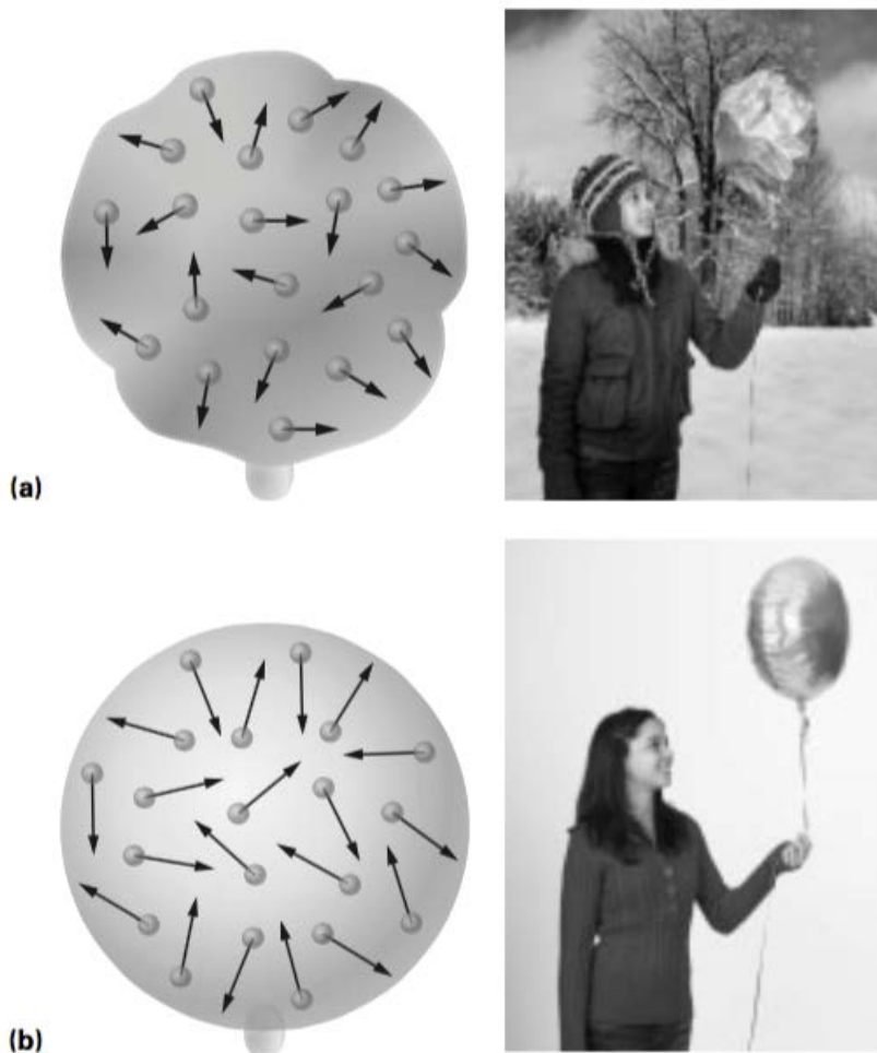
Figure 2 The helium gas in a balloon expands when you move a balloon from the cold outdoors to a warm room. (a) At a low temperature, the average kinetic energy of the particles in the balloon is low. The particles do not collide as often with the walls of the balloon, and hit the walls with less force. So, the balloon contracts. (b) As the temperature of the gas inside the balloon rises, the particles move faster and hit the wall of the balloon more often. So, the balloon expands.
