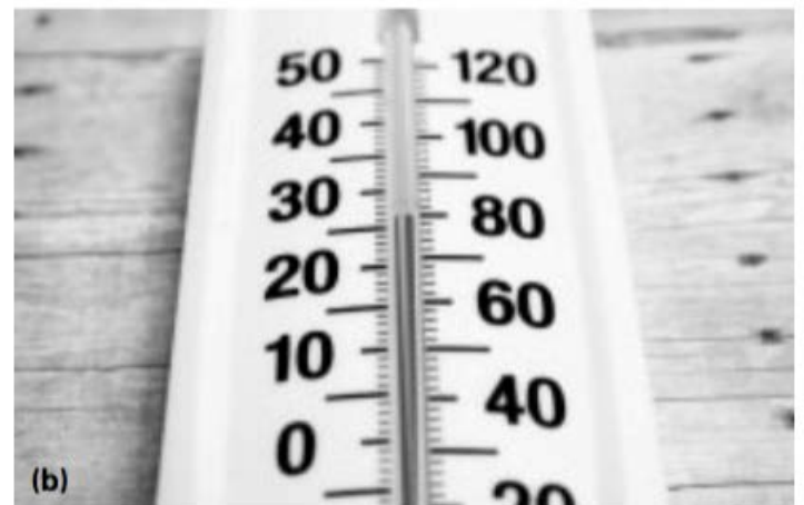
Figure 3 (a) Gasoline expands during hot weather. A full tank on a warm day could overflow. (b) The liquid in a thermometer expands and contracts as the air becomes warmer or cooler.
